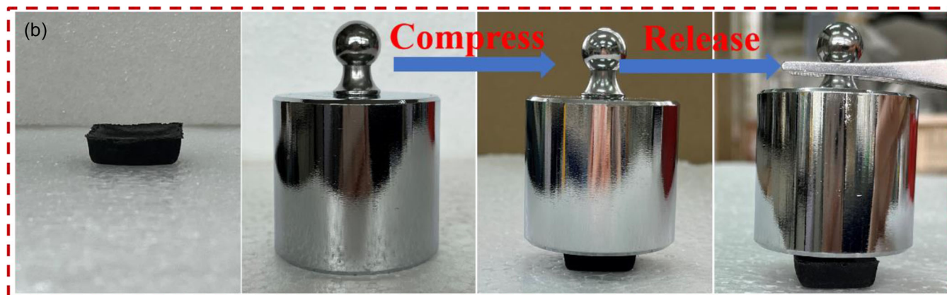
FIGURE 4 (a) Compressive stress–strain curves of PVA@LS, PVA@CLS, and PVA@PCLS; (b) PVA@PCLS with 500 g weight before and after bearing. LS, lignosulfonate; PCLS, porous LS-based biochar powder; PVA, polyvinyl alcohol.
