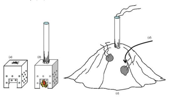
**Fig. 3.** Conventional, simple method for making rice husk charcoal. (*a*) A fire chamber is made from a tin can, the sides of which are pierced with small holes. (*b*) A fire is lit in the chamber, a chimney pipe is placed on top, and rice husks are heaped directly onto the unit. (*c*) When blackened husks appear on the surface of rice-husk mound, additional rice husks should be placed there. (*d*) Rice husks are carbonised inside of the mound.
