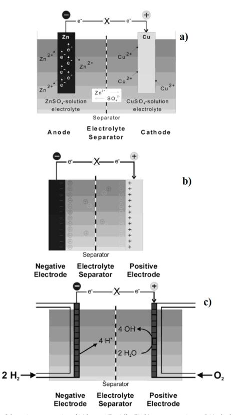
**Figure 5.** Schematic representation of (**a**) battery (Daniell cell), (**b**) a supercapacitor, and (**c**) a hydrogen fuel cell as reported by Winter et al. [219].
