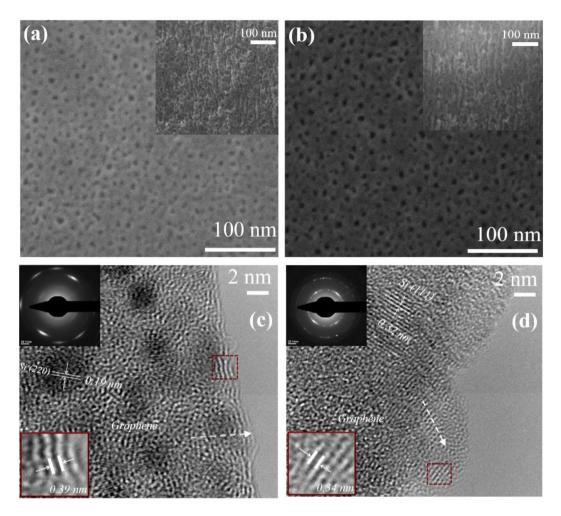
**Figure 1.** HR-SEM plan view images of modified porous silicon layer, corresponding to  $NC_J(\mathbf{a})$  and  $NC_CV(\mathbf{b})$  electrodes, respectively (cross-section detail – inset image); HR-TEM images of micropores for structure  $NC_J(\mathbf{c})$  and structure  $NC_CV(\mathbf{d})$ , respectively; upper inset: the corresponding SAED pattern.
