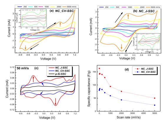
**Figure 3.** Cyclic voltammograms at different scan rates ranging from 5 to  $5000 \,\text{mV/s}$  for  $NC\_CV$ -SSC (a) and  $NC\_J$ -SSC (b) devices; (c) Comparative CV curves obtained at scan rates of  $50 \,\text{mV/s}$  with respect to reference p-Si-SSC; (d) Variation of SSC specific capacitance with the scan rate.
