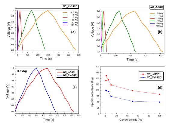
**Figure 4.** Charge discharge curves measured over the potential window of -0.9-1.2 V at different current densities ranging from 0.5 to 100 A/g for  $NC\_CV$ -SSC (a) and  $NC\_J$ -SSC (b) devices; (c) Comparative of the charge-discharge profiles measured at a constant current density of 0.5 A/g; (d) Variation of the specific capacitance with the current densities.
