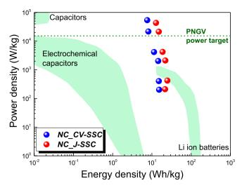
**Figure 6.** Ragone plots for *NC\_CV-SSC* and *NC\_J-SSC* devices.
