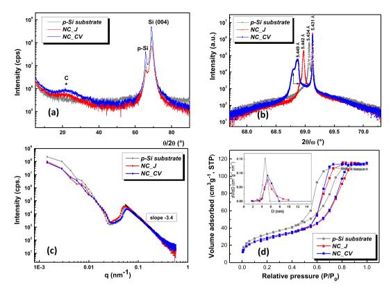
**Figure 2.** X-ray diffraction analyses: (a)  $\theta/2\theta$  wide angle X-ray diffraction; (b)  $2\theta/\omega$  scans for (004) Bragg reflections; (c) small angle X-ray scattering; and (d) N<sub>2</sub> adsorption/desorption isotherms for  $NC\_CV$  and  $NC\_J$  samples in comparison with p-Si substrate.
