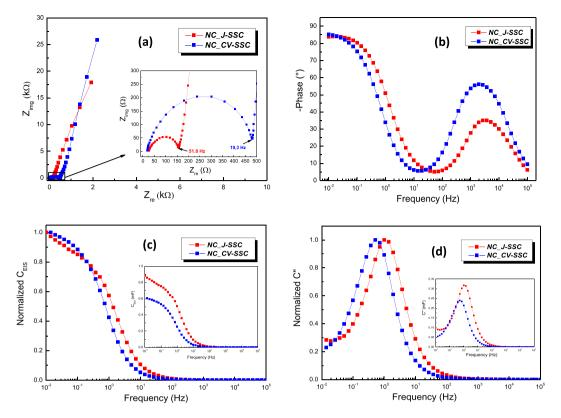
**Figure 5.** Electrochemical impedance spectroscopy measurements for  $NC\_CV$ -SSC and  $NC\_J$ -SSC devices: (a) Nyquist plots (inset: high frequency detail plots); (b) Bode phase angle plots as function of frequency; (c) variation of capacitance ( $C_{EIS}$ ) with frequency – normalized and absolute (inset) values; (d) variation of imaginary capacitance (C") with frequency – normalized and absolute (inset) values.
