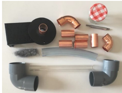
Fig. 4. Materials inventory for the construction of a thermoacoustic Stirling engine demonstrator.
