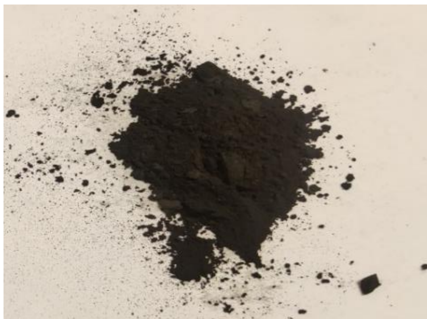
Fig. 7 Photograph of the graphite graphitized at 1300°C for 3 h with 22.4 wt% loading.
