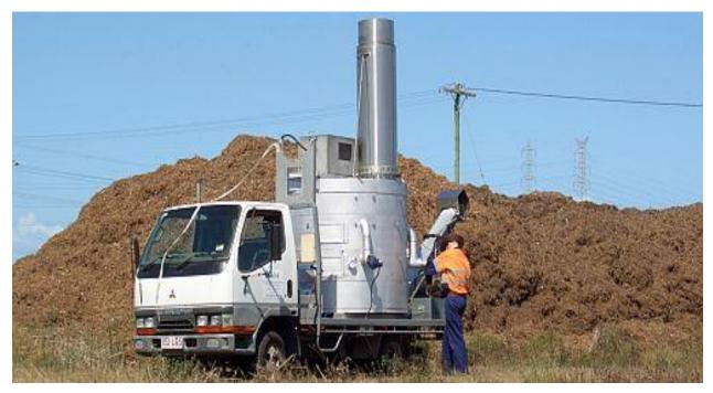
**Figure 60.** Mobile multiple-hearthfurnace commercialized by Black is Green Pty Ltd (<u>http://www.bigchar.com.au/about.html</u>, date accessed: Nov. 13, 2010).
