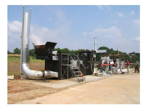
**Figure 67.** Picture of the torrefaction machine commercialized by Agri-Tech Producers, LLC (source: <u>http://www.agri-techproducers.com/</u>, date accessed: Nov. 13, 2010).
