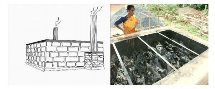
**Figure 43.** Improved Charcoal Production Systems (ICPS) or Adam retort (source: <u>http://www.biocoal.org/3.html</u>, date accessed: Nov. 15, 2010).
