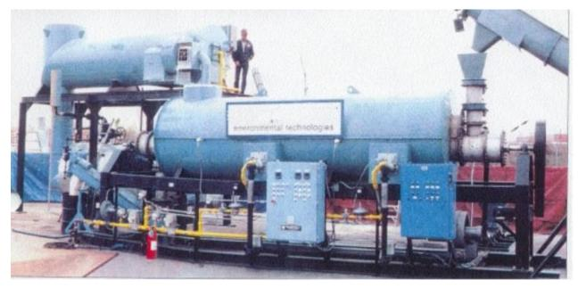
**Figure 68.** International Tech Corporation pyrolysis unit with heat recovery (<u>http://www.internationaltechcorp.org/IT-info.htm</u>, date accessed: Nov. 13, 2010).
