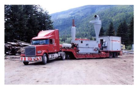
**Figure 23.** Mobile pyrolysis reactor developed by JF Biocarbon, Canada (source: <u>http://terrapreta.bioenergylists.org/taxonomy/term/1175</u>; date accessed: Nov., 15, 2010).
