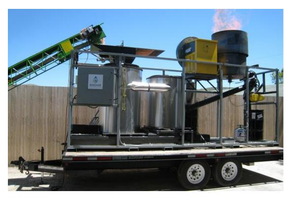
**Figure 58.** Picture of the mobile downdraft gasifier to produce biochar and heat from wood chips (source: <u>http://www.biocharengineering.com/technology/</u>, date accessed: Nov. 13, 2010).
