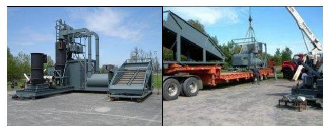
**Figure 22.** This 50 t/day portable (Mobile Pyrolysis Unit, ABRI) must be disassembled for transportation (source: <u>http://www.advbiorefineryinc.ca/home</u>; date accessed: Nov., 15, 2010).
