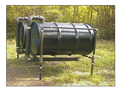
Figure 47. Small retort constructed of oil drums (<u>http://www.twinoaksforge.com</u> /BLADSMITHING /MAKING% 20CHARCOAL.htm, date accessed: Nov. 13, 2010).
