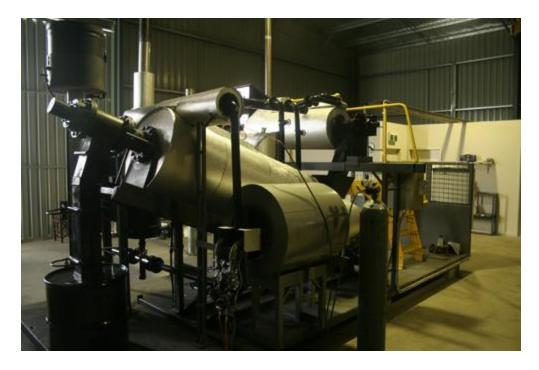
**Figure 69.** eGenesis CR-2 pyrolysis unit for the production of biochar and synthesis gases (<u>http://www.egenindustries.com/</u>, date accessed: Nov. 13, 2010).
