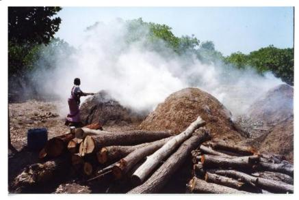
**Figure 25.** Earth kilns built in place (source: <u>http://www.biocoal.org/10.html</u>; date accessed: Nov., 15, 2010).
