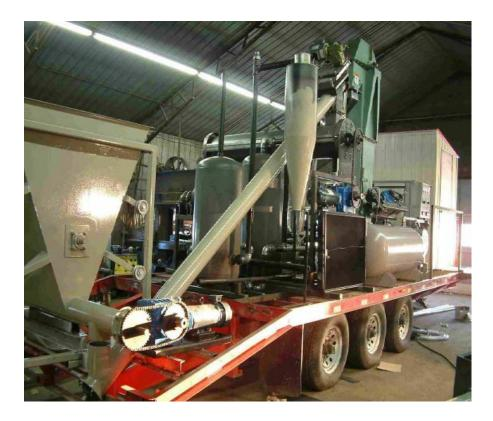
**Figure 65.** Renewable Oil International Mobile Unit using an auger pyrolysis reactor (Alabama USA).
