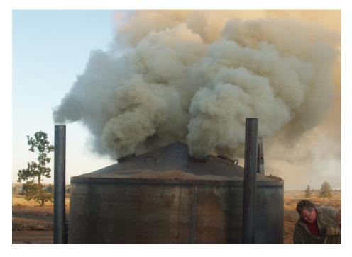
**Figure 2.** Environmental impact of carbonization units without recovery of volatile products (Courtesy of the Washington State Department of Ecology).
