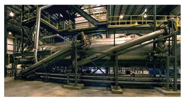
**Figure 70.** Moving bed system commercialized by NewEarth (<u>http://www.newearth1.net/e-oil.html</u>, date accessed: Nov. 13, 2010).
