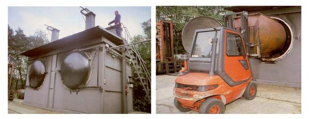
Figure 14. Semi-batch reactor - Van Marion Retort (VMR) system (source: <a href="http://www.bioforsk.no/ikbViewer/Content/71499/Biokarbonseminar%20%C5s%2011-03-2010%20Morten%20Gr%F8nli.pdf">http://www.bioforsk.no/ikbViewer/Content/71499/Biokarbonseminar%20%C5s%2011-03-2010%20Morten%20Gr%F8nli.pdf</a>) (date accessed: Nov., 14, 2010).
